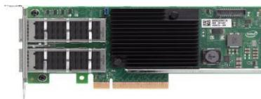
The Oracle Quad 10 Gb Ethernet Adapter or Oracle Dual 40 Gb Ethernet Adapter is one NIC that can be configured to either 10 GbE or 40 GbE.
